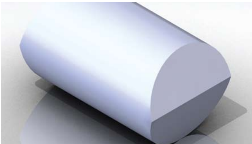
Fig. 7. Part design resulting from planar draft method.
