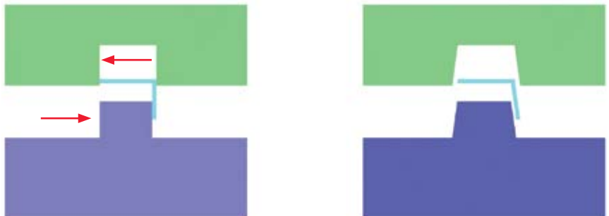
Fig. 3. Illustration shows the use of a telescoping shutoff without draft (left) and with draft (right). On the left, the arrows point to where tool wear will occur without drafting.
