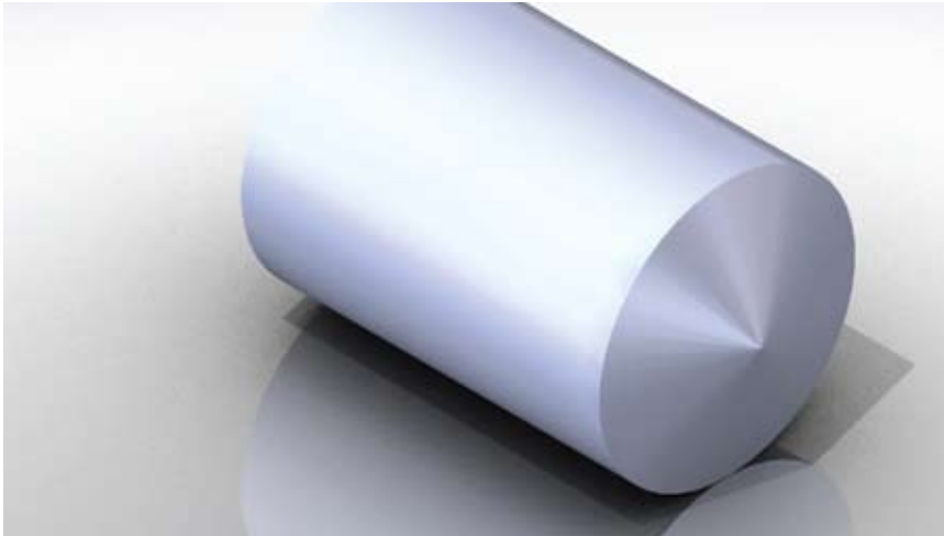
Fig. 6. Part design resulting from rotational draft method.
